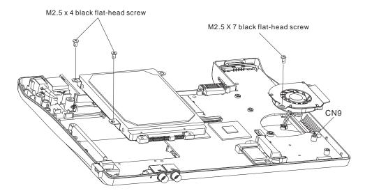
Figure 4-12 Removing the HDD pack
